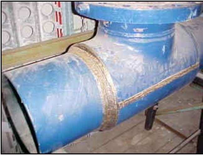
Fig. 1: Typical Split-tee in lab. Photograph: Gasunie.
