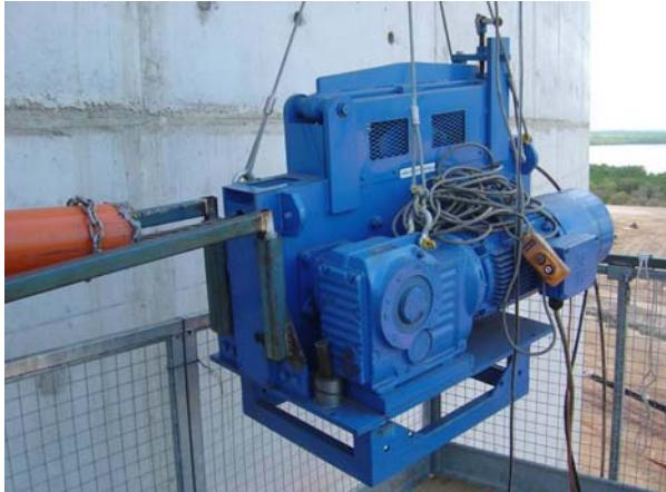
Figure 7 – High capacity strand pusher
