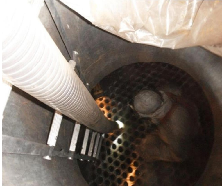
Figure 18: Loading of a tube reactor from the top. The flexible duct is the vacuum system for dust removal.
