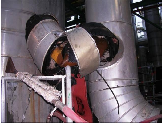
Fig. 2 – photo of the crease in pipe self-sealing the leak
