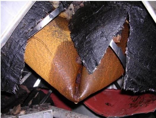
Fig. 2 – photo of the crease in pipe self-sealing the leak
