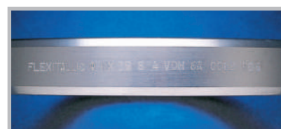
Low stress stamping for identification and traceability
