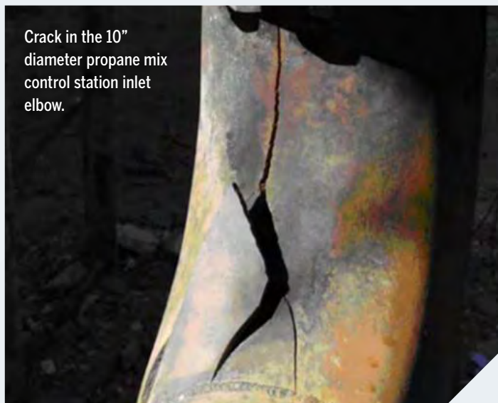
A dead-leg is a section of piping connected to the process that has no flow through it.
